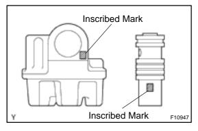
If necessary, replace the flow control valve with the one having the same letter as inscribed on the rear housing.
