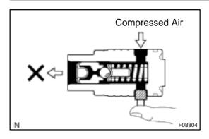
(b) Check the flow control valve for leakage. Close one of the holes and apply compressed air of 392 − 490 kPa (4 − 5 kgf/cm², 57 − 71 psi) into the opposite side hole, and confirm that air does not come out from the end hole.
