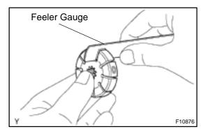
Inscribed Mark F10878 If it is more than the maximum, replace the vane plate and/or vane pump rotor with the one having the same mark stamped on the cam ring.
